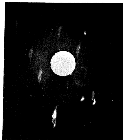
FIGURE 29. Asterism. Gold at 493^{\circ}\text{C} : ( a ) unstrained, ( b ) glide 13 %. Silver at -180^{\circ}\text{C} : ( c ) unstrained, ( d ) glide 35 %, ( e ) glide 54 %. Compare figure 12, curve 1 of which refers to this crystal.
